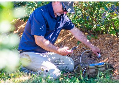
**The HydraGO and HydraGO FLEX** system features a rugged, Delran housing that contains a rechargeable battery. The internal battery will last for long field sessions with repeated and frequent data samplings.
